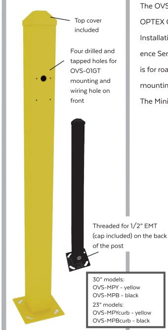
The OVS-MP is a sturdy Mini Post specially designed for the OPTEX OVS-01GT and OVS-01CC Vehicle Presence Sensors. Installation is easy with the OVS-MP. The Vehicle Presence Sensor mounts at the proper height. The 30" model is for road surfaces, and the 23" model is for island or curb mounting. No more ground loops, no more concrete cutting. The Mini Post is Powder Coated, tougher than paint.
