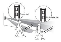
3 Set the DIP switch 1 (WALK TEST MODE) to "OFF (NORM)".
