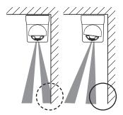
When the unit is mounted on the corner to look ahead along the wall, choose the guide-mark located on the opposite side of the wall.
