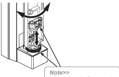
Check that the fixture and bracket engage correctly.
