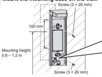
Use this knockout screw hole to mount the base, when making the wall tamper switch effective. If the main unit is peeled off from a wall, this plastic part will be cracked and remain on a wall, activating the tamper switch.
