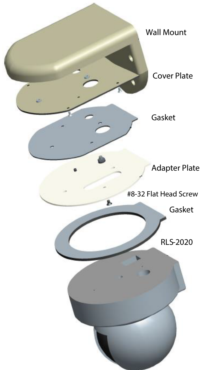
Figure 2 - 2020-WMA8 exploded view
